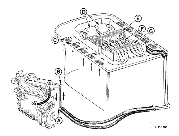
A-Supply hose (from cylinder block) B-Return hose (to water pump) C-Air intake openings D-Fan E-Radiator (or radiator and evaporator) F-Air recycle filter G-Air filter
