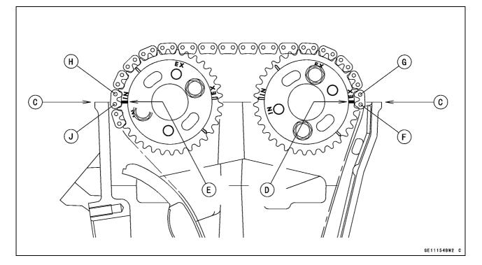
• Install the camshaft cap, while pushing the camshaft chain, tighten all camshaft bolts and chain guide bolts.
