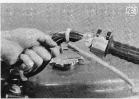
Loosen the front brake adjusting nut and pull the cable off the brake lever. (Expansion brake models)
