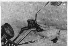
Loosen the handlebar mountings, remove the right upper mount, move the handlebar to the left for easy cable removal, and tighten the left mounting.
