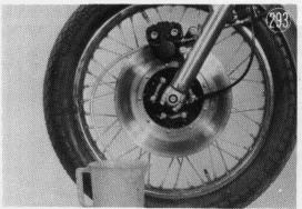
•Open the bleeder valve, squeeze the brake lever, close the valve, release the lever. Repeat this sequence several times until the hose is full of fluid.
