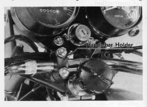
Screw in the throttle and starter cable adjusters completely to give the cables plenty of play.
