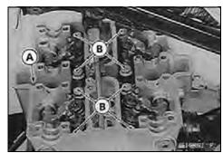
• Tap in the places shown with a mallet [A] to remove the cylinder head.
