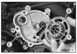
Position the idle gear [A] to inside of the mating surface
