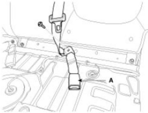
Fig. 15: Identifying Seat Belt Buckle (LH) Courtesy of KIA MOTORS AMERICA, INC.
