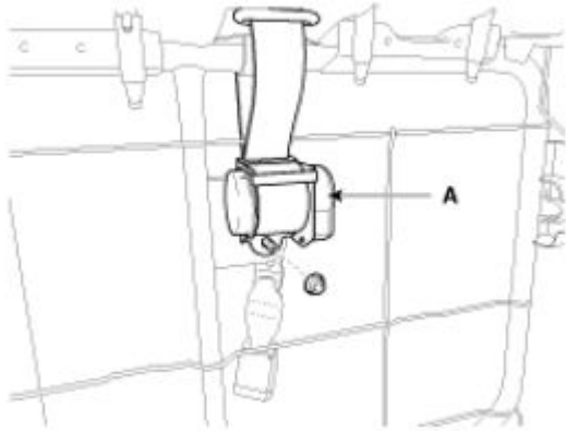
Fig. 14: Identifying Seat Belt Center Retractor Courtesy of KIA MOTORS AMERICA, INC.
