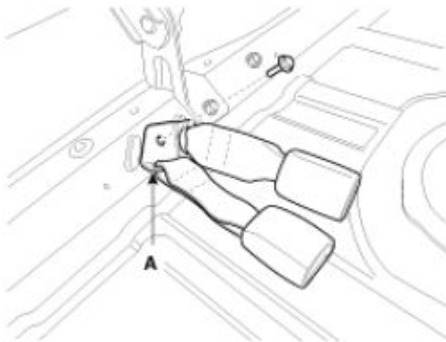
Fig. 16: Identifying Seat Belt Buckle (RH) Courtesy of KIA MOTORS AMERICA, INC.
