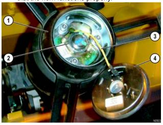
FIGURE 5-3. STEERING WHEEL RETAINER NUT
