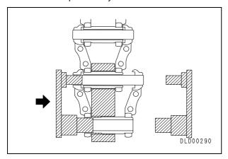
Return the left cylinder and operate the right cylinder to pull out the pin and bushing press-fitting portion from the right link simultaneously.
