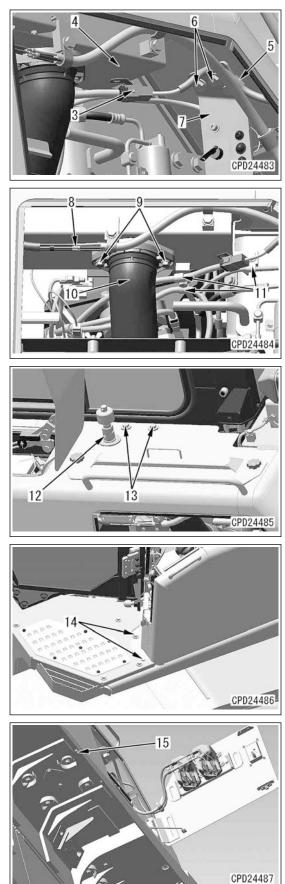
12. Close cover (2), and remove it from parts (a) (3 places) of battery cover (4) by using the nylon sling.
