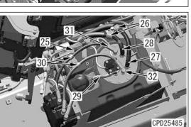
• After disconnecting the AdBlue/DEF hose, install tool H to the hose side and install tool J to the nipple side to prevent leakage.
