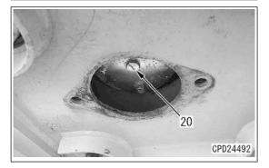
25. When the AdBlue/DEF tank becomes empty, install drain plug (20) securely.
