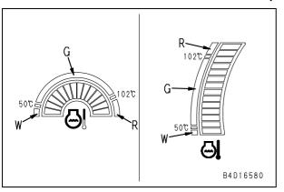
★ Power train oil temperature: Max. range Serial No.: 30001 – 30131 Serial No.: 30132 and up
