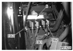
A In order to prevent malfunction and mistaken system error warning, be sure to completely remove foreign object (b) such as sand, dust, water, etc., from inside of controller side connector (a) with air blow etc., before connecting to harness connector.
