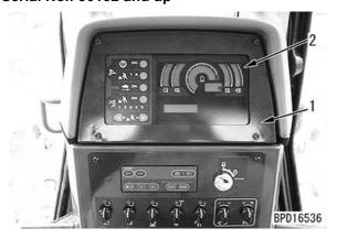
Insert or connect T-adapters in or to connectors S01, S02, S03, and S04 of machine monitor (2).
