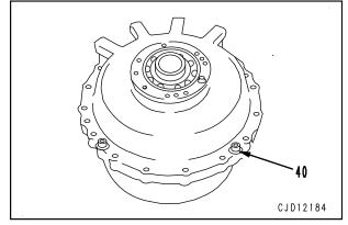
8. Installation of brake and carrier assembly
