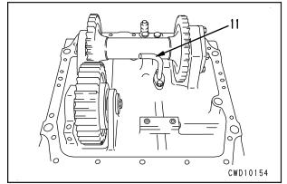
4) Input gear assembly1] Install bearing (10) to gear (9).
