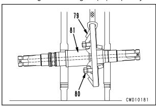
$\star$  Tighten mounting nut (80) temporarily.
