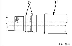
Insert bevel gear shaft (81) into bevel gear (79) being lifted at the case center from the right side of the machine.
