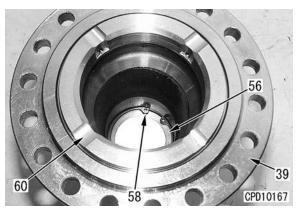
3) Install hub (39) to hub (54) and tighten 18 bolts.
