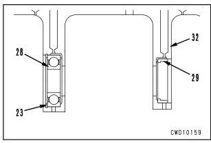
4] Press fit shaft (21) to the inner race side of bearing (28).
