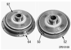
7) Install hub and carrier assembly (64) to hub (54) and install bolt (89).
