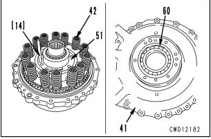
14)Using eyebolt [15], align cover (41) with the guide bolt and set it.
