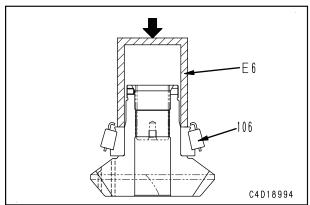
2] Use tools **E7** and **E8** to press fit outer race (105) and (107) into cage (103).
