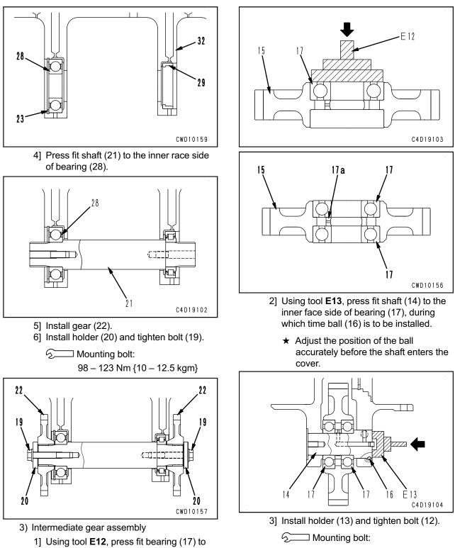
gear (15) and install spacer (17a).
