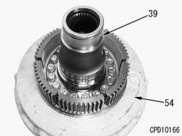
4) Install bearing (57) to hub (39). 5) Install snap ring (59).
