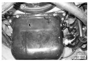
13. Pull oil pan (13) forward until it can pass main cap (14) of No. 6 engine cylinder.
