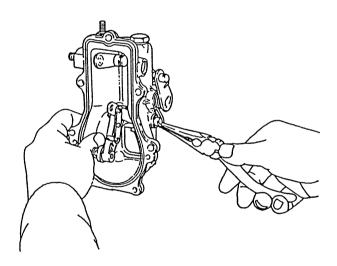
(10) Hook the governor spring on the control lever shaft and tension lever hook with long nosed pliers.
