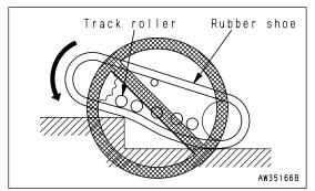
2) Furthermore, if the machine travels in reverse, a gap is formed between the track roller, idler, and rubber shoe.
