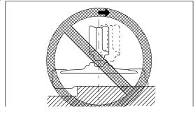
• If the machine is turned in this condition, the rubber shoe will come off.
