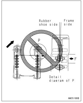
• If the machine travels in reverse in this condition, the rubber shoe will come off.
