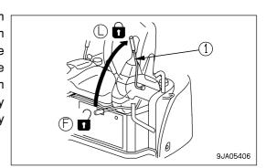
When leaving the machine, always lower the work equipment and blade completely to the ground, set lock lever (1) to LOCK position (L), then stop the engine. Use the key to lock all the equipment. Always remove the key, take it with you, and keep it in the specified place.
