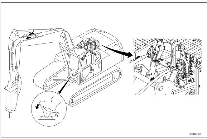
When the front of the pedal is depressed, oil flows to the piping on the left side of the work equipment; when the rear of the pedal is depressed, oil flows to the piping on the right side of the work equipment. (When a breaker is installed, only the front of the pedal can be used.)
