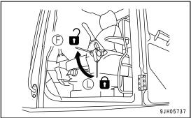
4. Set the lock lever to LOCK position (L).
