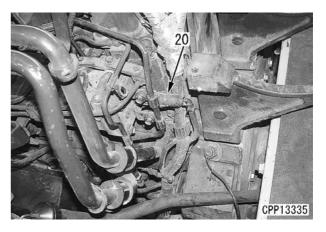
15. Remove clamp (23), bolts (24) and bracket (25) to remove the housing complex (diffuser) (26).
