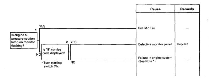
Note 1: The monitor panel display has returned to normal, but the engine oil pressure Hi sensor has detected symptoms of a drop in the oil pressure in the past, so carry out troubleshooting of the engine to remove the problem.
