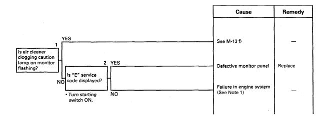
Note 1: The monitor panel display has returned to normal, but the air cleaner clogging sensor has detected symptoms of clogging in the past, so carry out troubleshooting of the engine to remove the problem.
