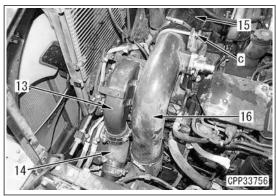
46. Fasten MIKALOR clamps at both ends of hose (14) according to the following procedure.
