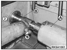
C. Lubricate the threading and the first part of the cylinder (2).
