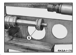
G. Mount the nut (5) that secures the piston and tighten it with the socket wrench **E** and the dynamometric tool with a multiplier **D**.
