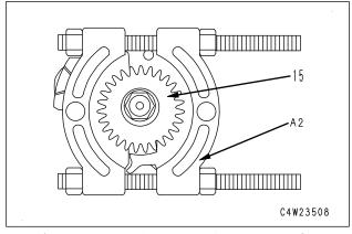
3) Install puller [2] on tool A2 and the shaft.
