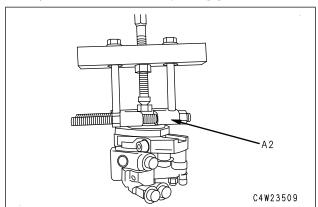
6) Remove nut (14), lock washer (18) and gear (15) from shaft (17).
