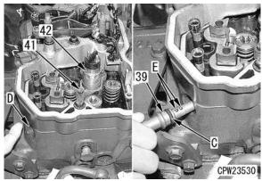
9) Tighten mounting bolts (41) of holder (40) alternately.
