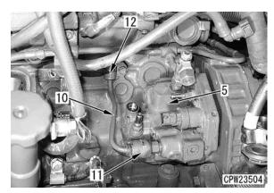
12.Remove nuts (13) (3 places), and remove supply pump (5). [\*3]
