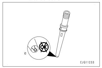
7) Apply engine oil to O-ring (part C) and head side (part D) of inlet connector (39).
