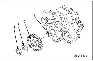
3. Use support A1 and 1/2-inch spin handle [1] to fix the gear, and tighten nuts (14).
