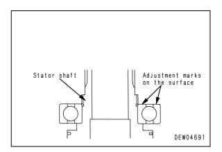
8) Using tool C2, install nut (24) to stator shaft.
