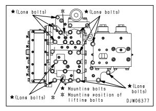
Using eyebolts [1] (Dia. = 10 mm, Pitch = 1.5 mm), lift off control valve assembly (3).
