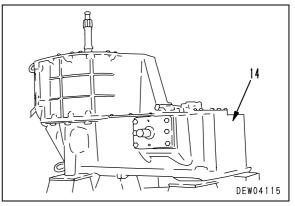
Using eyebolts [4] (Dia. = 16 mm, Pitch = 2.0 mm), lift off transmission case (15).
