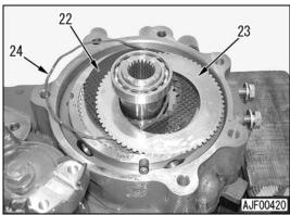
★ Soak the discs in clean transfer oil for at least two minutes before installing them.
