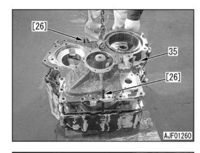
C. Install snap ring (86) on the HST motor 2 side.
