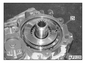
B. Install seven discs (22), seven wave springs (24), and eight plates (23).
