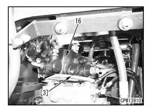
18. Lift steering demand valve assembly (21) again and remove it.
