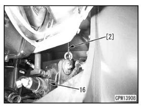
16. Remove mounting bolt (17) for steering demand valve assembly (16).
