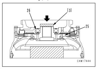
4) Remove mounting bolt to separate turbine (27) and boss (25).
