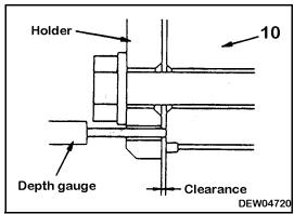
F. Insert shim and rotate cage while tightening holder mount bolts to specified tightening torque.
