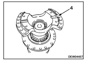
★ Rotate the cage 20 - 30 times, then using push-pull scale ①, check the starting torque.
