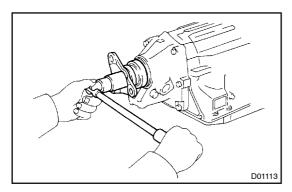
(b) Using a deeper socket wrench of 30 mm, remove the nut.
