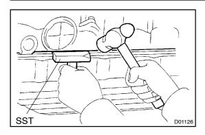
(b) Insert the blade of SST between the transmission case and oil pan, cut off applied sealer.
