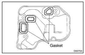
(c) Remove the 3 gaskets from the oil strainer.
