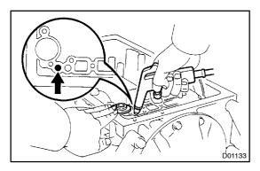
(e) Applying compressed air to the oil hole, remove the  $C_0$  accumulator piston and spring.
