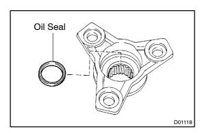
(d) Remove the oil seal from the output flange.
