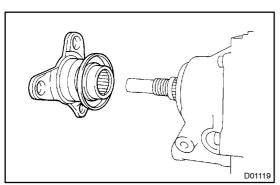
(c) Remove the output flange.
