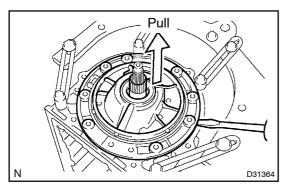
(b) Using screwdriver, pull out the oil pump.
