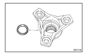
(c) Remove the oil seal from the flange yoke assy.
