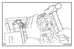
(b) Using a pin punch and a hammer, drive out the spring pin. HINT:
