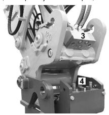
Fig. 18 LIKUFIX during coupling
