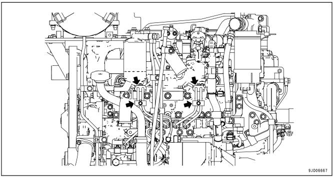
Check visually and touch by hand to check that there is no hardening of the rubber and no loose bolts of the mounting clamps (4 places) for the high-pressure piping between the supply pump and the common rail. If there are any problems, the parts must be replaced. In this case, please ask your Komatsu distributor to carry out replacement. Replacement of the high-pressure piping must be made as an assembly.
