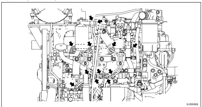
The fuel spray prevention caps (12 places) on the fuel injection piping and both ends of the high-pressure piping act to prevent the fuel from coming into contact with high-temperature parts of the engine and causing a fire if the fuel should leak or spray out. Check visually and touch by hand to check that there are no missing caps, loose bolts or hardening of the rubber. If there are any problems, the parts must be replaced. In this case, ask your Komatsu distributor for replacement.
