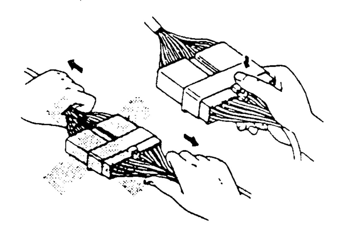
Connectors can be disconnected by pressing or pulling the lock lever as shown.
