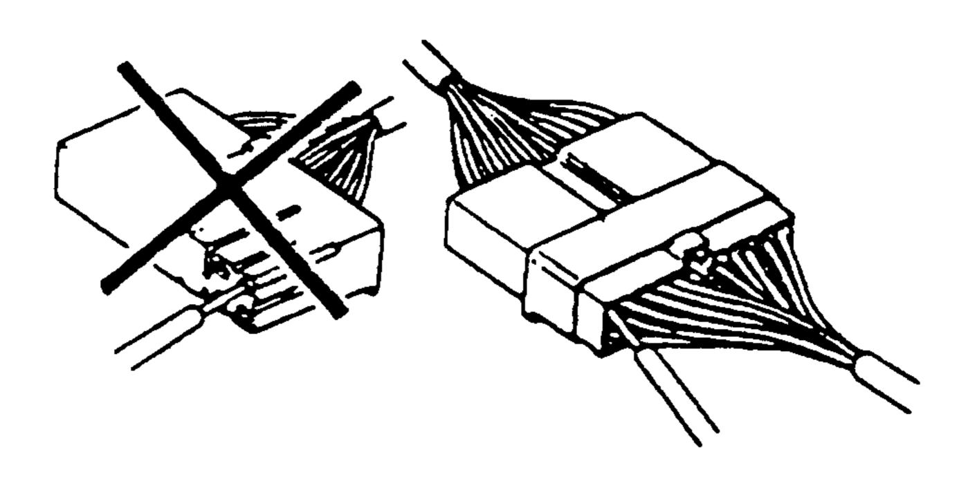
2. Check the terminals of waterproof connectors from the connector side, as they cannot be accessed from the wiring harness side.
