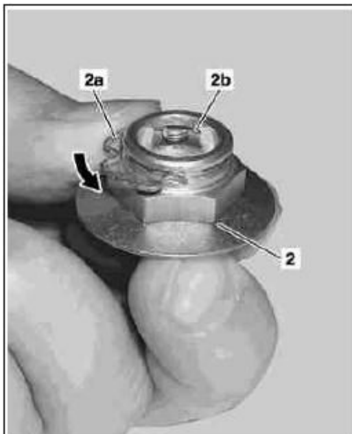
Fig. 4: Pushing Retaining Clamp Courtesy of MERCEDES-BENZ USA
