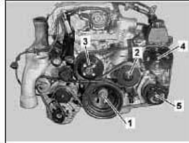
Fig. 21: Running Diagram Of Poly V-Belt (Engine 111.955 With AC Compressor)
