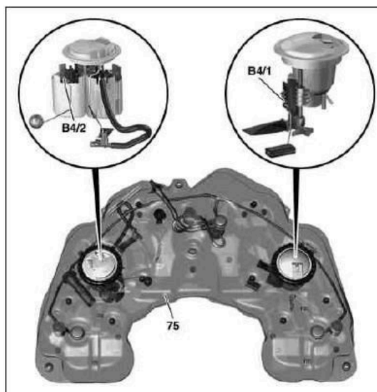
Fig. 2: Locating Fuel Level Sensors - Except Model 216, 221 Courtesy of MERCEDES-BENZ OF NORTH AMERICA.
