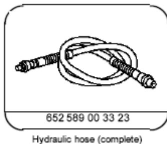
Fig. 26: Identifying Hydraulic Hose (Complete) (652 589 00 33 23) Courtesy of MERCEDES-BENZ OF NORTH AMERICA.
