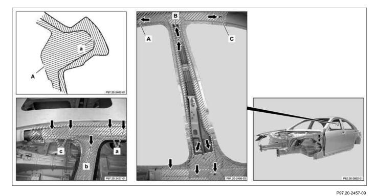
B-pillar on longitudinal member, outer side paneling and inner roof frame
