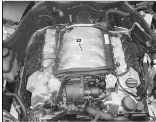
Fig. 5: Identifying Variable Intake Manifold - Engine 113.988 Courtesy of MERCEDES-BENZ USA
