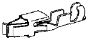
Fig. 25: Identifying Junior Power Timer (JPT) Pin Courtesy of MERCEDES-BENZ OF NORTH AMERICA.
