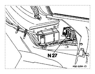
Model 126 N27 Anti-tow trigger unit
