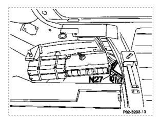
Model S 124 N27 Anti-tow trigger unit
