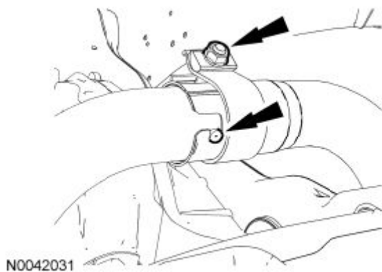
Fig. 1: Locating Muffler Assembly-To-Tail Pipe Torca® Clamp Courtesy of FORD MOTOR CO.
