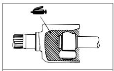
Grease: repair kit grease Amount used: 110 ± 10 g
