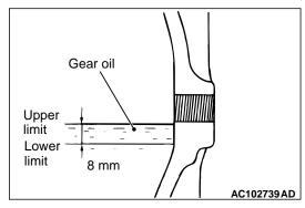
Check that gear oil level is not 8 mm below the bottom of filler plug hole.
