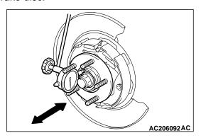
2. Fit the dial gauge as shown in the diagram and move the hub in the axial direction to measure the play.
