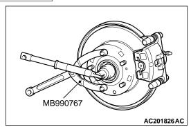
Do not apply pressure to wheel bearing by the vehicle weight to avoid possible damage to wheel bearing before tightening drive shaft nut fully.
