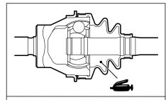
Grease: repair kit grease Amount used: 75 ± 10 g
