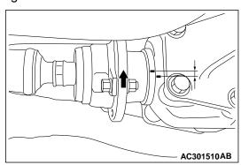
4. Turn the propeller shaft counterclockwise as far as it will go, and measure the amount of distance between the mating marks.
