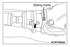
3. Turn the propeller shaft clockwise as far as it will go. Make the mating marks on the companion flange and on the differential carrier.
