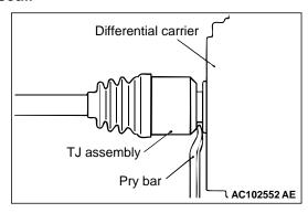
2. Remove the drive shaft from the differential carrier by using a pry bar.
