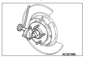
5. Measure to determine whether the wheel bearing axial play is within the specified limit or not.
