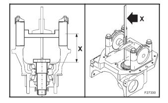
In order to determine the necessary thickness value (S) between the pinion and the bearing, subtract the value (V), stamped on the pinion head (V = requested conical distance), from the measured value (X).
