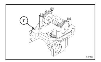
Assembly diagram of the "false differential box" tools **380000407** + **380000440** on the bearing differential support seats.
