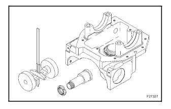
Insert the bearing (3) and (8) in their housings. Assemble the "false pinion" **380002219** and its ring nut (10).
