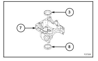
To remove the bearing (3) of the bevel pinion (1), use a standard extractor.
