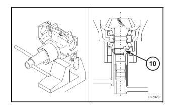
Remove the ring nut (10) and collect its retaining washer (9).
