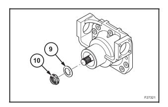
Tap the shaft with a soft hammer to remove the bevel pinion (1).
