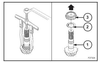
Check all pinion components for wear.
