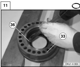
Remove bearing outer cup (35) from flange (33).
