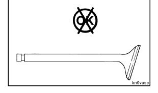
Measure the rim thickness to determine if there is enough stock to grind the valve.
