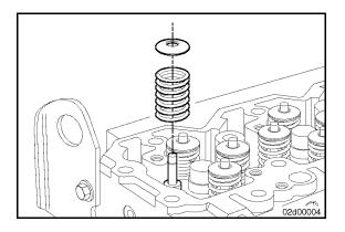
Release valve spring and remove the spring retainer and spring.
