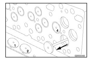
Remove the remaining collets, retainers, springs and valves.
