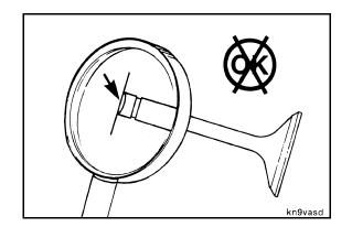
Inspect for bent valves.
