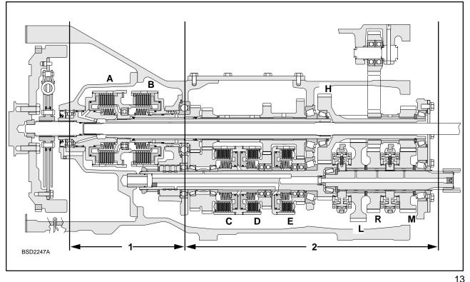
The SEMI–POWERSHIFT transmission is subdiviced into a speed (1) and range (2) sections providing 6 speed gears in each of 3 ranges:–
