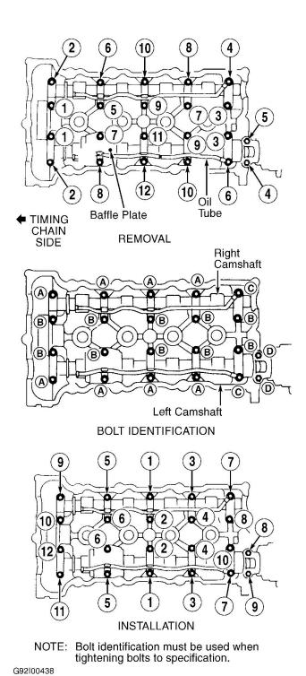
Fig. 19: Camshaft Bearing Cap Bolt Identification & Removal & Installation Sequence Courtesy of NISSAN MOTOR CO., U.S.A.
