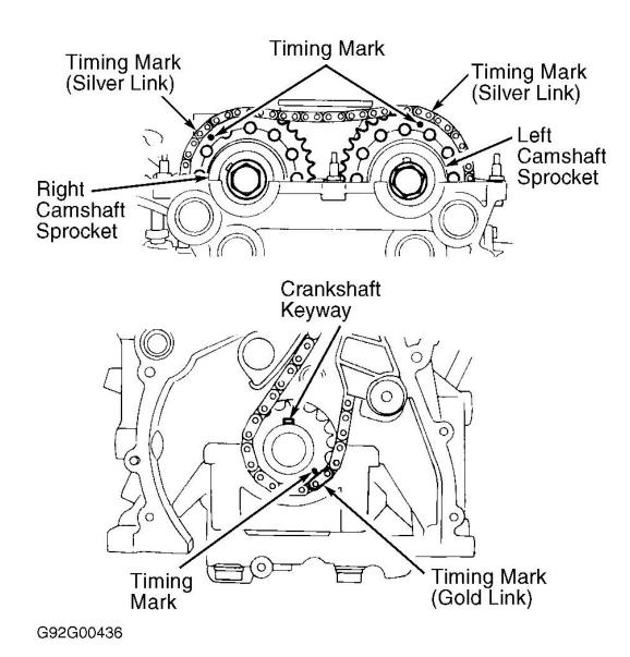
Fig. 17: Aligning Timing Marks
