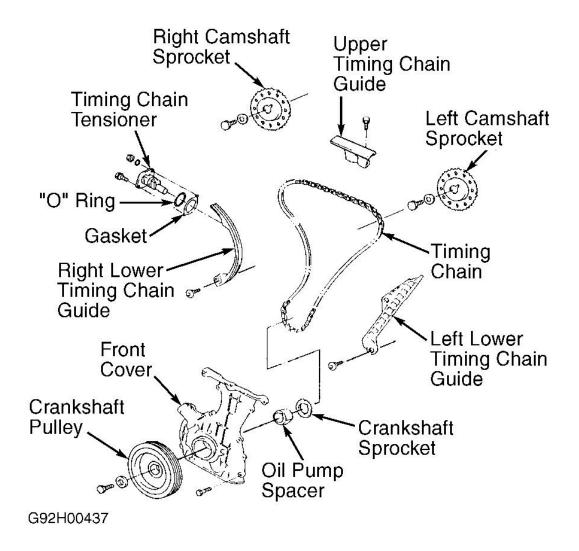
Fig. 18: Exploded View Of Timing Chain & Components Courtesy of NISSAN MOTOR CO., U.S.A.
