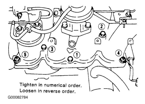
Fig. 9: Intake Manifold Plenum Tightening Sequence Courtesy of NISSAN MOTOR CO., U.S.A.
