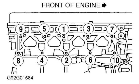
Fig. 8: Intake Manifold Tightening Sequence (Altima, Frontier & 240SX) Courtesy of NISSAN MOTOR CO., U.S.A.
