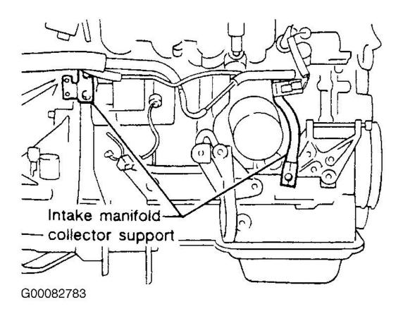
Fig. 7: Identifying Intake Manifold Plenum Supports Courtesy of NISSAN MOTOR CO., U.S.A.
