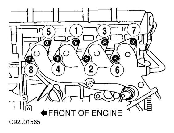
Fig. 10: Exhaust Manifold Tightening Sequence (Altima, Frontier & 240SX) Courtesy of NISSAN MOTOR CO., U.S.A.
