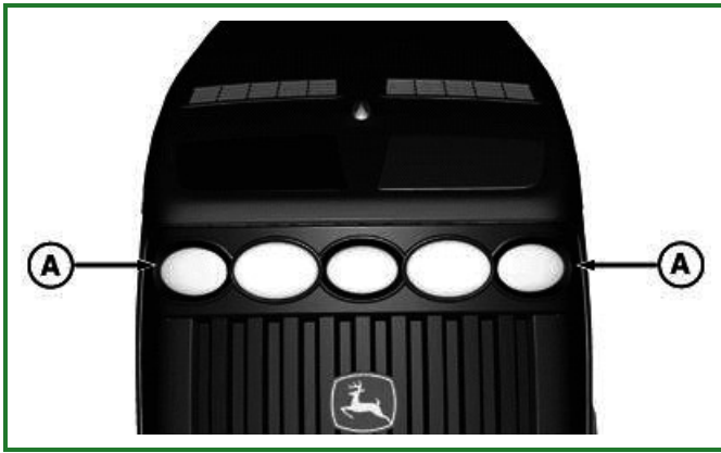
RXA0080172-UN: Pull Front Bezel Straight Back
