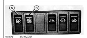
Press switch (A) to turn on heater.
