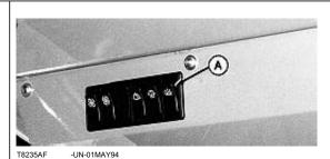
Press switch (A) to turn dome light ON.
