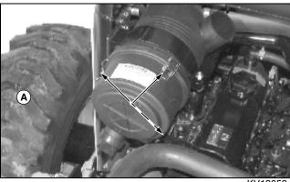
4. Unhook three end cap latches (A) and remove end cap.
